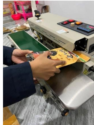
Gambar II - 8 Proses sealer kemasan
